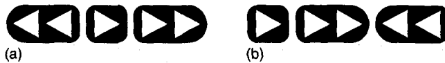
Figure 1.9 (a) Natural mapping between rewind, play, and fast forward on a tape recorder device. (b) An alternative arbitrary mapping.
