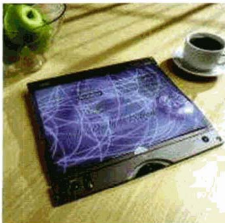
(ii) an IBM prototype of a color electronic ink page, is intended for e-newspapers that can 'typeset' themselves and update while being light enough to carry around.
