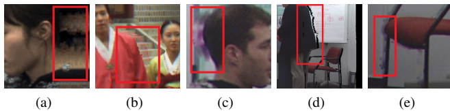
Fig. 2. Distortions introduced by DIBR techniques, which are mainly located around the dis-occlusion regions (dominant distortions are highlighted by red bounding boxes).
