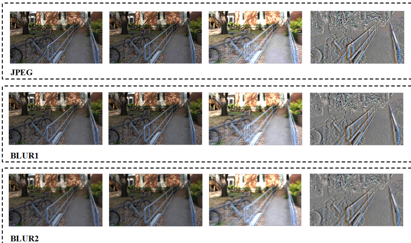
Fig. 2: Examples of distorted stereoscopic images with different distortion types/levels and the corresponding fusion as well as difference maps. JPEG distorted stereoscopic image (top), low-degree BLUR (i.e. BLUR1) distorted stereoscopic image (middle) and high-degree BLUR (i.e. BLUR2) distorted stereoscopic image (bottom). The first to the last columns show left view images, right view images, fusion maps and difference maps, respectively.
