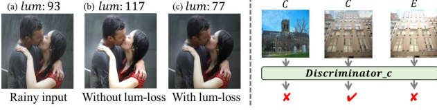
Figure 5. Left: directly using the real clean images (usually sunny in dataset) to constraint the de-rained outputs often causes over-bright results (b) and don’t match the cloudy situation (c). Right: by enhancing luminance in clean images \{c_j\}_{j=1}^M \in C , we additionally generate a negative training sample set E : \{e_k\}_{k=1}^K \in E .
