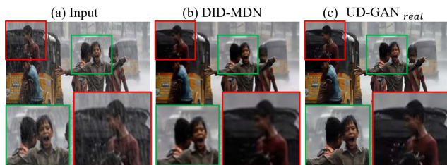
Figure 6. UD-GAN real that trained only on real rainy data shows a little bit lower PSNR (around 0.4dB) compared with other supervised methods on synthetic datasets, but achieves much better subjective results for real-world rainy images. As shown above, the details of the boy’s face and the car’s logo have been clearly preserved in result (c), compared with DID-MDN’s blur result (b).
