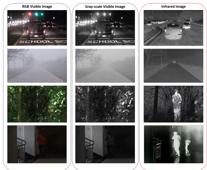
Fig. 1. An illustration of differences between infrared and visible images. This figure gives some examples for visible RGB-scale, visible gray-scale, and infrared images taken under the same conditions, i.e. with light pollution, bad weather, severe occlusion, and darkness. We can see that visible images may show more details, while infrared ones are more temperature-sensitive, and more robust to bad conditions.
